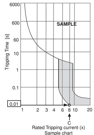
C : Multiple of tripping current at tripping time 0.01s
