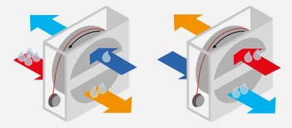
Key component is the enthalpy wheel, made with alternatively flat and corrugated aluminum sheets.
