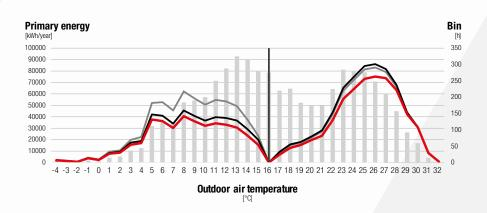
The energy analysis displays how i-FX-N heat pump is always more convenient if compared with the other two solutions.
