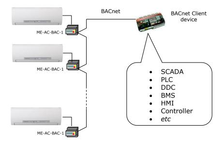
The ME-AC-BAC-1 interface allows a complete and natural integration of *Mitsubishi Electric* air conditioners into either BACnet IP or MS/TP networks. Compatible with Domestic (RAC), Mr Slim and City Multi line models commercialized by MITSUBISHI ELECTRIC.
